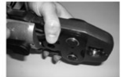
Вставьте пресс-тиски в инструмент, а крепежный болт в пазы. Place the pressfitting jaw in the machine and insert the fastening bolt until it fits.
